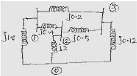
4. For the network shown in fig. form the bus admittance matrix. Determine the reduced admittance matrix by eliminating node 4. (16)
