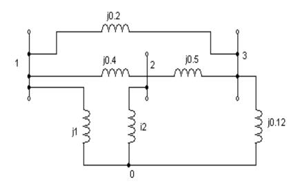
10. Using Singular transformation method, Determine YBUS for the network shown in Fig. Where the impedance labeled in p.u (16)
