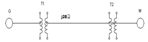
6. The single line diagram of an unloaded power system is shown in Fig. The generator transformer ratings are as follows.
