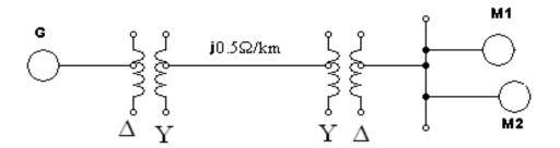
5. Draw the reactance diagram for the power system shown in Fig. Use a base of 50 MVA 230 kV in 30  $\Omega$  line. The ratings of the generator, motor and transformers are:
