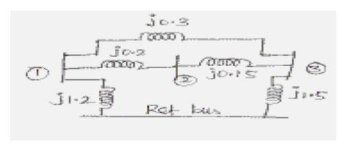
3. Using building algorithm method, determine ZBUS for the network shown in Fig where the impedances are labeled are shown in per unit. (16)
