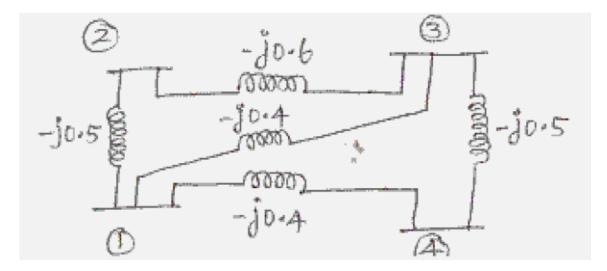
5. Using building algorithm method, determine  $Z_{\text{BUS}}$  for the network shown in Fig. where the impedances are in p.u.
